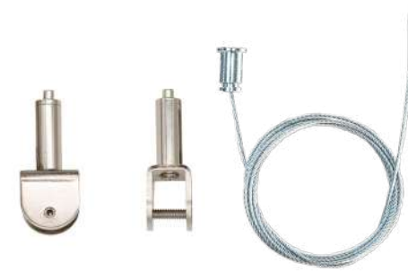
Anchor C to hang 9-12 mm thickness suspended panel with steel cable. Adjusted included (from 150 mm to 2000 mm).
